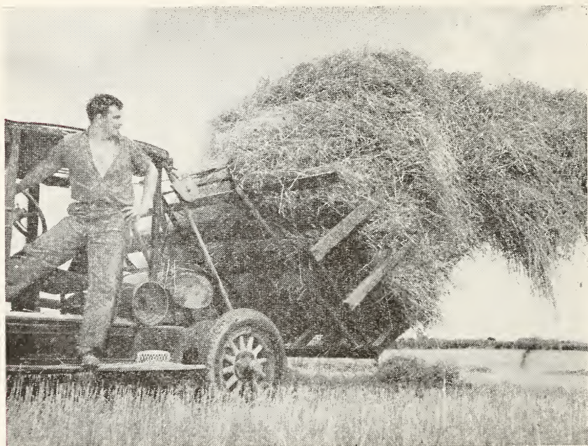
FIGURE 10.—A typical auto buckrake made from parts of an old automobile. In this picture straw is being hauled. Performance of this type of buckrake is practically the same as that for tractor buckrakes. However, an auto buckrake generally represents more of an investment than does a tractor buckrake as the tractor is not considered a part of the outfit.
